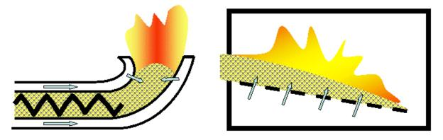
Since the burner is fed from below, using a screw, and the screw feed must be designed so as to prevent back-firing (i.e. that the flames creep backwards through the screw) the feed will be dimensioned as narrow as possible. Hence, the fuel feed will not allow larger or more porous particles to pass and a pellet burner becomes fuel inflexible.
