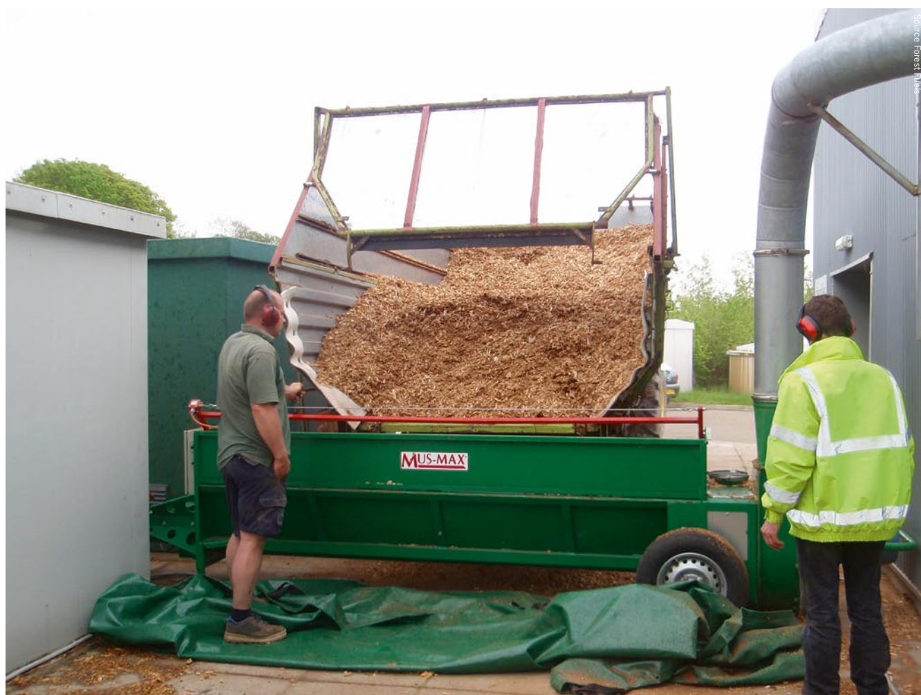
Mus-max blower, useful for transferring woodchip fuel upwards or into awkward spaces, noise, additional power supply, slow delivery rate resulting in increased costs are potential pitfalls with this approach.
