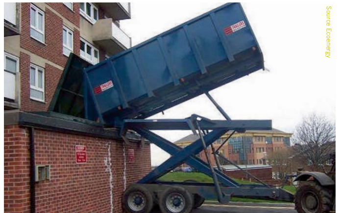
Woodfuel bunker with hydraulic lids, fuel is delivered using a high "scissor lift" trailer.
