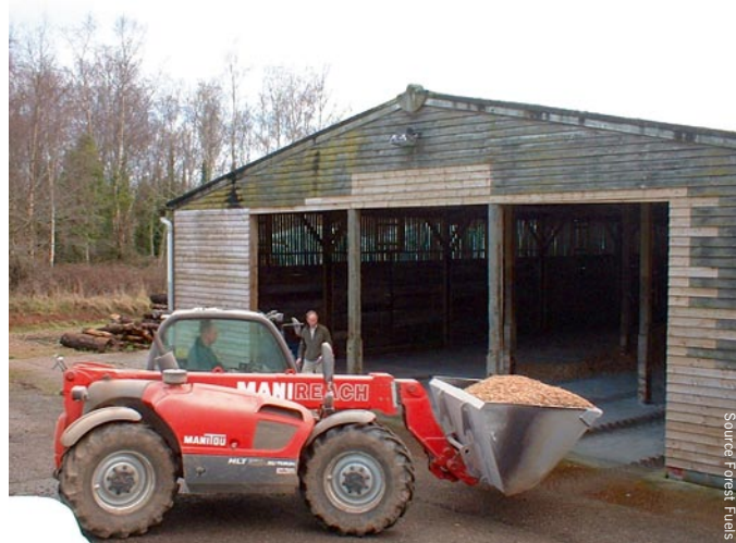
Loading barn stored G30 chip at 19% moisture content for delivery.
