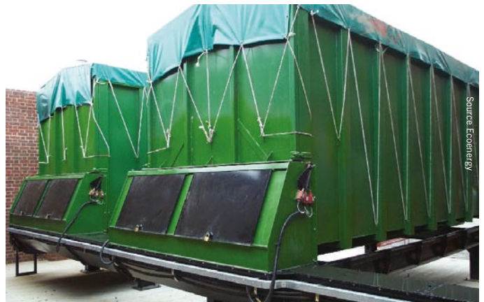
Dual 35 cubic metre hookbin fuel delivery system
