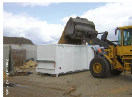
Hook bin being loaded at distribution depot – loading bucket with a capacity of 5 cubic metres, less than 5 minutes to load a 20 cubic metre bin
