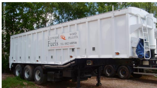
Pellet Tanker for blown delivery – body compartmentalised to allow for partial delivery.
