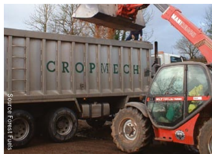
Eight wheeler being load with finished chip – vehicle volume 28 cubic metres
