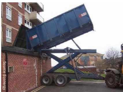
Scissor lift trailer – specialised trailer for high lift tipping cost circa £15 – 20,000
