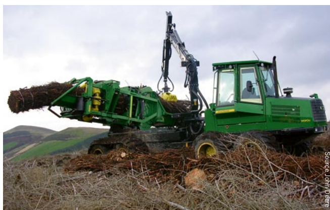
Baler producing log bundles of harvesting brash, ready for transportation and then chipping
