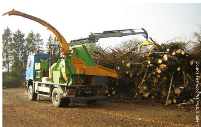
Holzhack Chipper 14-800 purpose built lorry mounted chipper with seven metre reach grab—working with whole trees at roadside
