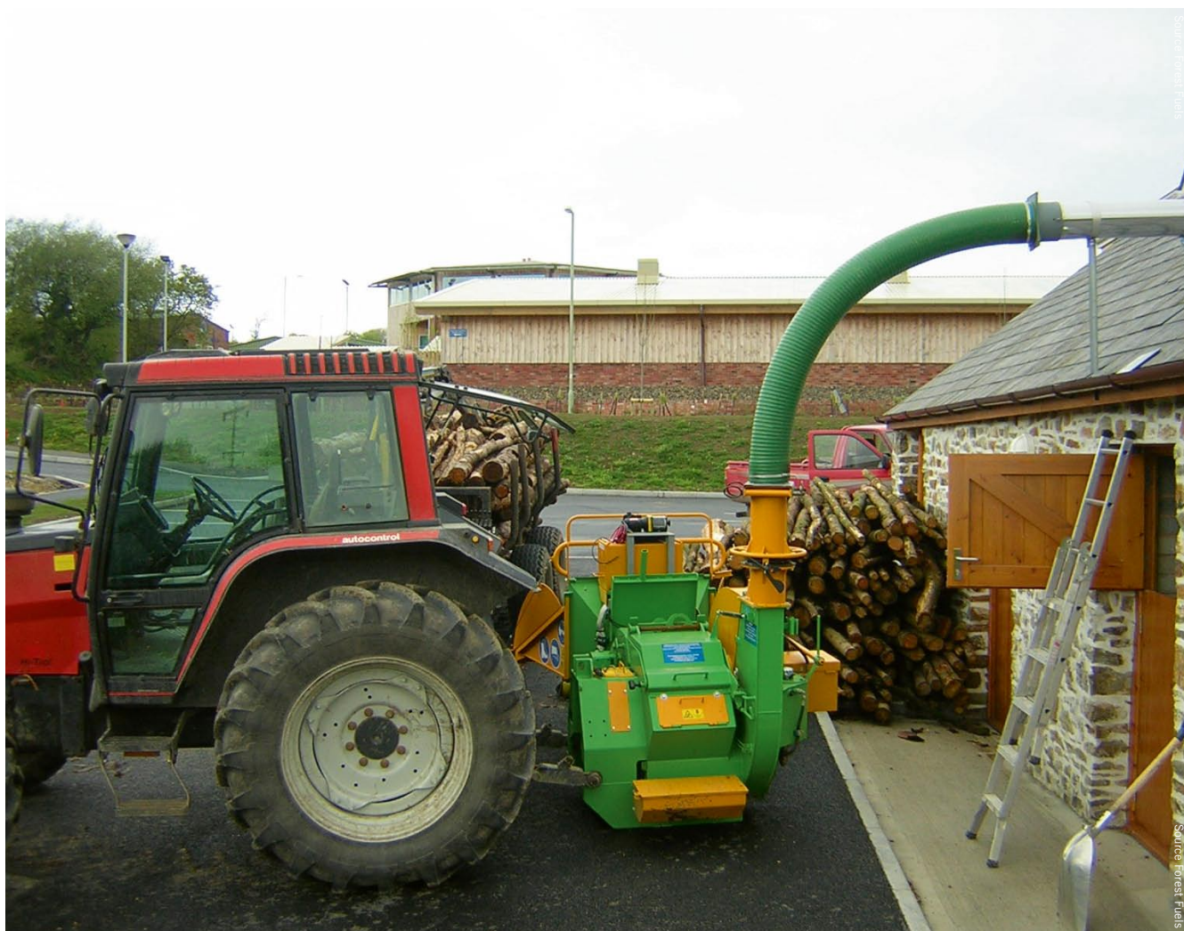
Direct chipping into fuel store – useful option where noise of chipping and timber storage is acceptable or as in this case where no other option is available due to limited delivery access via pedestrian door.
