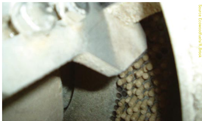
Khal pellet press and die with emerging pellets
