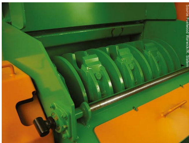
Internal view of drum chipper showing blade settings.
