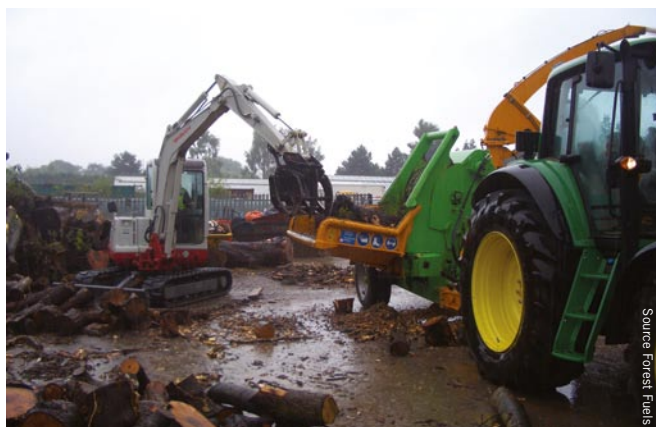
Excavator feeding chipper with arboricultural arisings of all shapes and sizes which would be difficult to crane feed with a conventional timber grab. Oxford City Council Tree Station
